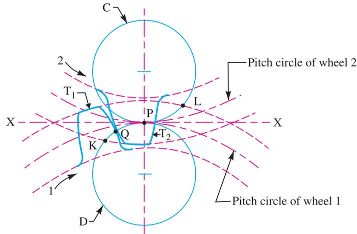
Fig. 28.9. Construction of two mating cycloidal teeth.
