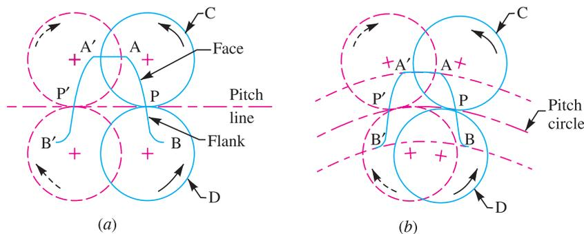
**Fig. 28.8.** Construction of cycloidal teeth of a gear.
