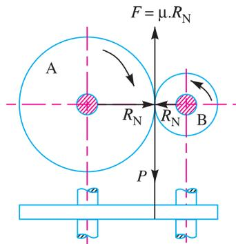
Fig. 28.1. Friction wheels.
